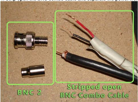
2. Slip on the crimping part of the BNC2 Connector, making sure the inner metal conduct inserts correctly into the BNC female.
