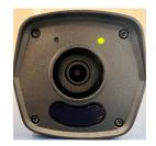
Flashing Red LED. Move Camera closer to NVR. Out of Range
