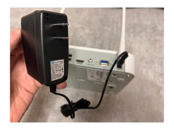
Each camera will need its own power source. Connect the 12VDC 1A power supply to each camera you wish to add to your SV-WK4-N wireless kit.
